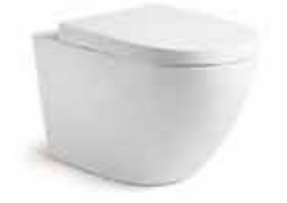
SY1014F • Back to wall toilet • Size : 555*365*800mm • P-trap: 180mm roughing in • S-trap: 120/150mm roughing in
