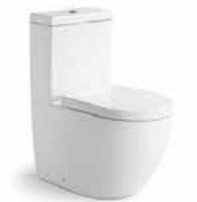
SY8831 • Washdown one-piece toilet • Size : 670*370*840mm • S-trap: 250mm roughing in • P-trap: 180mm roughing in
