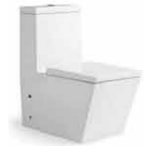
SY389 • Siphonic / Washdown one-piece toilet • Size : 665*355*820mm • Siphonic / S-trap: 300/400mm roughing in • Washdown / S-trap: 250mm roughing in • P-trap: 180mm roughing in
