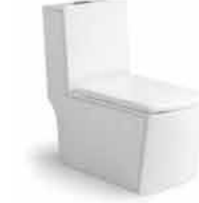
SY3958 • Washdown one-piece toilet • Size : 710*380*820mm • S-trap: 300/400mm roughing in • P-trap: 180mm roughing in
