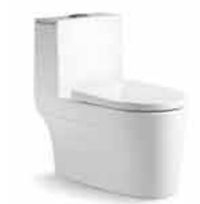
SY3971 • Siphonic / Washdown one-piece toilet • Size : 680*400*790mm • Siphonic / S-trap: 300/400mm roughing in • Washdown / S-trap: 250mm roughing in • P-trap: 180mm roughing in
