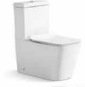
SY8869 • Washdown one-piece toilet • Size : 660*360*800mm • S-trap: 250mm roughing in • P-trap: 180mm roughing in
