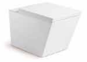
SY1001F • Back to wall toilet • Size : 555*355*800mm • P-trap: 180mm roughing in • S-trap: 100mm roughing in
