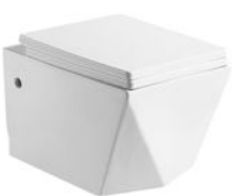
PL-7809 Rimless wall hung toilet Size:520x360x370mm P-trap 180mm roughing-in
