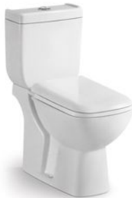
PL-6615 Washdown two-piece toilet Size: 650x370x795mm P-trap 180mm roughing-in S-trap 250mm roughing-in
