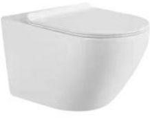
PL-7791 Rimless wall hung toilet Size:485x360x365mm P-trap 180mm roughing-in
