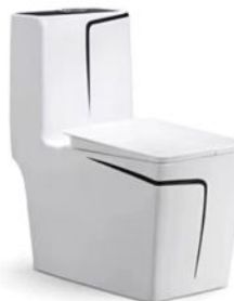
PL-3890-B Siphonic/Washdown one-piece toilet Size:685x355x775mm Siphonic/S-trap:250/300/400mm roughing-in Washdown/P-trap:180mm roughing-in
