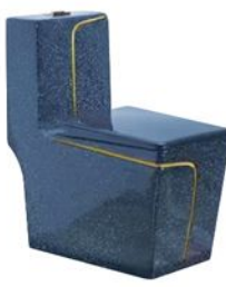
PL-3890-1 Siphonic/Washdown one-piece toilet Size:685x355x775mm Siphonic/S-trap:250/300/400mm roughing-in Washdown/P-trap:180mm roughing-in
