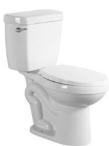
PL-6070 Siphonic two-piece toilet Size:740x460x750mm S-trap 300/400mm roughing-in
