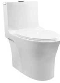
PL-3003 4D Super swirling one-piece toilet Size:720x385x700mm S-trap 300/400mm roughing-in
