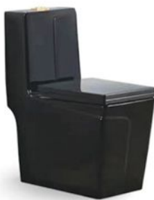
PL-3890-Q Siphonic/Washdown one-piece toilet Size:680x355x780mm Siphonic/S-trap:250/300/400mm roughing-in Washdown/P-trap:180mm roughing-in
