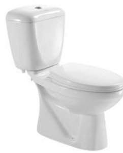
PL-6823 Washdown two-piece toilet Size:695x385x750mm S-trap 250mm roughing-in P-trap 180mm roughing-in
