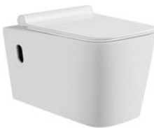
PL-7836 Rimless wall hung toilet Size:575x355x375mm P-trap 180mm roughing-in
