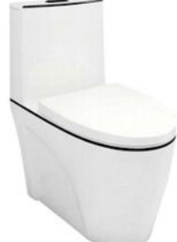
PL-3806-E Siphonic/Washdown one-piece toilet Size:650x370x780mm Siphonic/S-trap:250/300/400mm roughing-in Washdown/P-trap:180mm roughing-in
