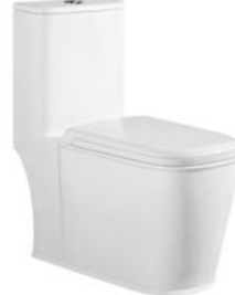
PL-3864 Washdown one-piece toilet Size:750x400x860mm S-trap 250mm roughing-in P-trap180mm roughing-in
