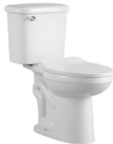
PL-6177 Siphonic two-piece toilet Size:735x370x770mm S-trap 300/400mm roughing-in
