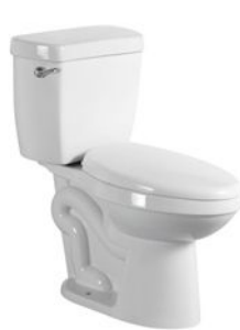
PL-6071 Siphonic two-piece toilet Size:735x370x770mm S-trap 300/400mm roughing-in
