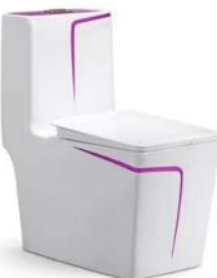
PL-3890-0 Siphonic/Washdown one-piece toilet Size:685x355x775mm Siphonic/S-trap:250/300/400mm roughing-in Washdown/P-trap:180mm roughing-in
