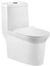
PL-3002 2D Super swirling one-piece toilet Size:740x380x760mm S-trap 300/400mm roughing-in
