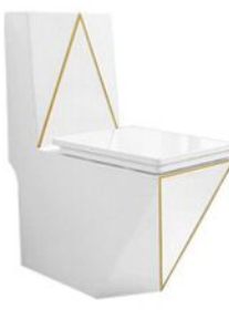
PL-3814-F Siphonic/Washdown one-piece toilet Size:680x370x830mm Siphonic/S-trap:250/300/400mm roughing-in Washdown/P-trap:180mm roughing-in
