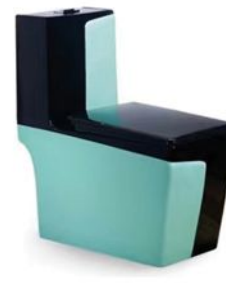
PL-3890-Z Siphonic/Washdown one-piece toilet Size: 685x355x775mm Siphonic/S-trap: 250/300/400mm roughing-in Washdown/P-trap: 180mm roughing-in
