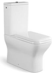
PL-6066 Washdown two-piece toilet Size: 640x350x840mm P-trap 180mm roughing-in S-trap 250mm roughing-in
