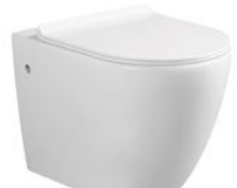
PL-7770 Siphonic wall hung toilet Size:550x360x385mm P-trap 180mm roughing-in
