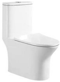
PL-3216 2D Super swirling one-piece toilet Size:660x370x760mm S-trap 300/400mm roughing-in
