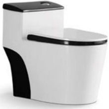
PL-3328-A Siphonic/Washdown one-piece toilet Size:700x390x630mm Siphonic/S-trap:250/300/400mm roughing-in Washdown/P-trap:180mm roughing-in
