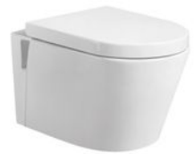
PL-7708 Washdown wall-hung toilet Size:560x360x350mm P-trap 180mm roughing-in
