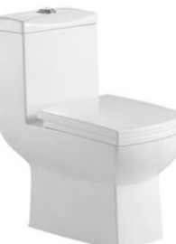
PL-3830 Siphonic one-piece toilet Size:660x350x770mm S-trap 220/250/300mm roughing-in P-trap 180mm roughing-in
