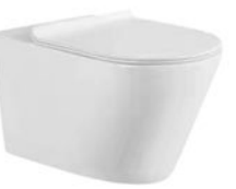
PL-7792 Rimless wall hung toilet Size:490x360x365mm P-trap 180mm roughing-in
