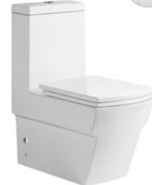
PL-3859 Washdown one-piece toilet Size:660x350x750mm S-trap 250mm roughing-in P-trap180mm roughing-in
