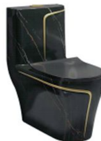
PL-082 Siphonic/Washdown one-piece toilet Size:710x380x750mm Siphonic/S-trap:250/300/400mm roughing-in Washdown/P-trap:180mm roughing-in
