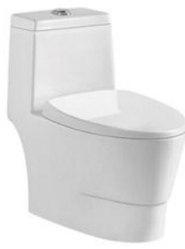
PL-3808 Washdown&Siphonic one-piece toilet Size:690x390x710mm S-trap 250/300mm roughing-in P-trap180mm roughing-in
