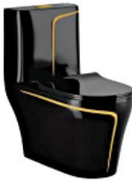
PL-3899-J Siphonic/Washdown one-piece toilet Size:710x380x750mm Siphonic/S-trap:250/300/400mm roughing-in Washdown/P-trap:180mm roughing-in
