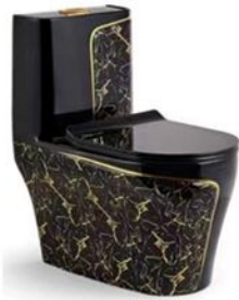
PL-285BCG Siphonic/Washdown one-piece toilet Size:690x390x740mm Siphonic/S-trap:250/300/400mm roughing-in Washdown/P-trap:180mm roughing-in
