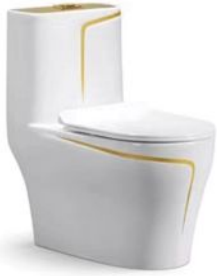
PL-3899-L Siphonic/Washdown one-piece toilet Size:690x390x740mm Siphonic/S-trap:250/300/400mm roughing-in Washdown/P-trap:180mm roughing-in
