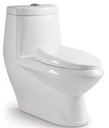
PL-3882 Washdown one-piece toilet Size: 745x415x720mm P-trap 180mm roughing-in S-trap 250mm roughing-in
