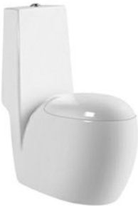
PL-3884 Washdown one-piece toilet Size:730x365x900mm S-trap 250mm roughing-in P-trap 180mm roughing-in
