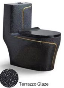
PL-3899-4 Siphonic/Washdown one-piece toilet Size:690x390x740mm Siphonic/S-trap:250/300/400mm roughing-in Washdown/P-trap:180mm roughing-in
